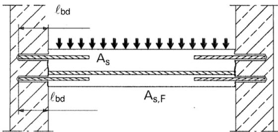
**Figure A5:** Anchoring of reinforcement to cover the line of acting tensile force
