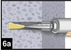
6. Starting from the bottom or back of the cleaned bore hole fill the hole with adhesive, until the level mark at the mixer extension (see below) is visible at the top of the hole. For embedment larger than 190 mm an extension nozzle shall be used. Slowly withdraw the static mixing nozzle and using a piston plugs during injection of the mortar, helps to avoid creating air pockets.
