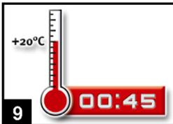
9. Observe gelling time  $t_{gel}$ . Attend that the gelling time can vary according to the base material temperature (see Table B3). Do not move or load the bar until full curing time  $t_{cure}$  has elapsed (attend Table B3).
