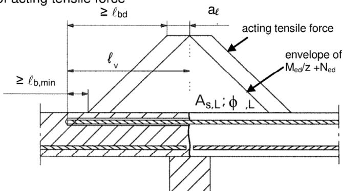
**Figure A2:** Overlapping joint at a foundation of a wall or column where the rebars are stressed in tension
