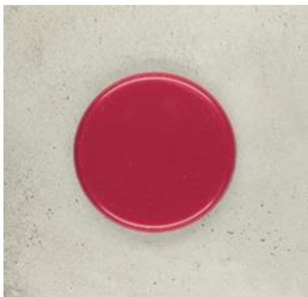
Figure 1: HIT-RE 500 V4 cured without contact to air; background: concrete
