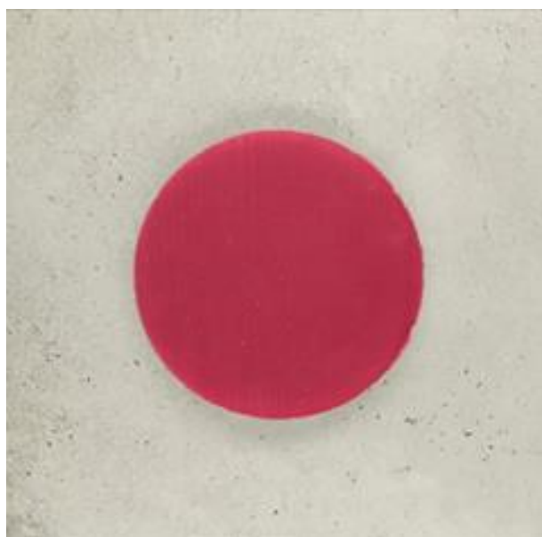
Figure 2: HIT-RE 500 V4 cured with contact to air; background: concrete
